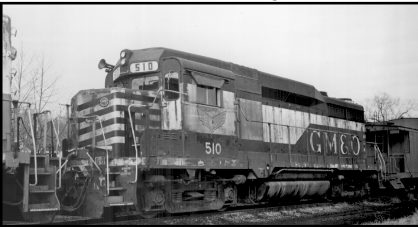
ICG (GM&O) GP30, looking a bit on the ratty side, sits on the ready track at the Central City, KY engine facility. Note the Alco trucks. January 7, 1984 Photo by Chuck Hinrichs
